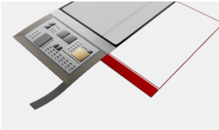
Light blocking in LCD backlight unit
