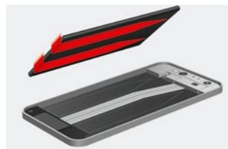
Battery mounting in mobile devices
