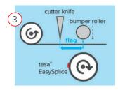
Make sure that the flag is approximately as long as the distance between the bumper/contact roller and the knife. This will help to have the best bond between two webs.
